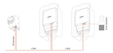
7.2.2 Charger(s) and LMC connected via CAN. All devices connected to web via wifi or 4G. Last charger on the line to be equipped with end resistor to provide reliable communication between devices.
